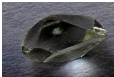
Figure 3. Single crystal of obtained CaTT
